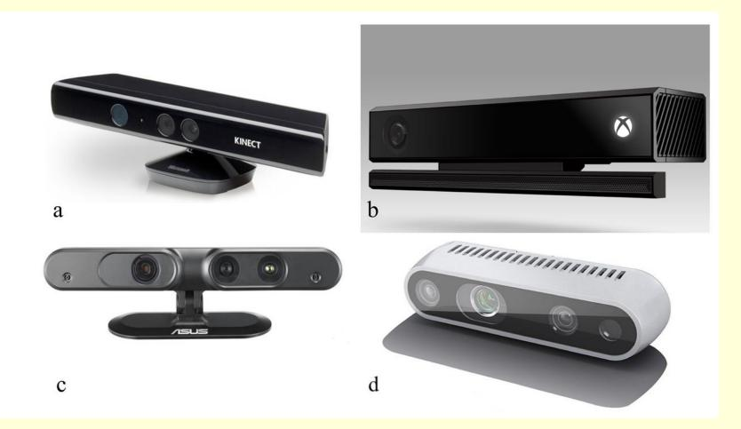
RGB-D cameras: a - Microsoft Kinect v1, b - Microsoft Kinect v2, c - Asus Xtion PRO LIVE, d - Intel RealSense D435
