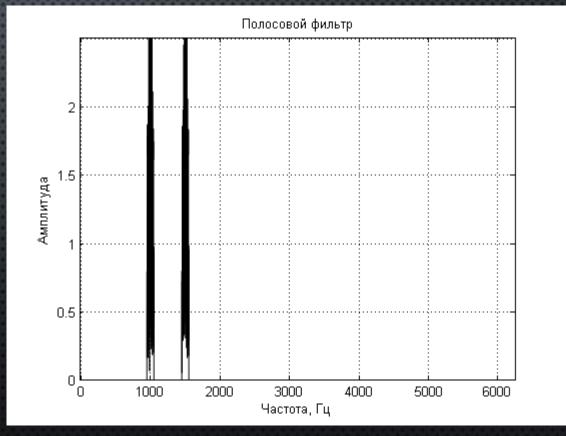
The spectrum of the filtered signal
